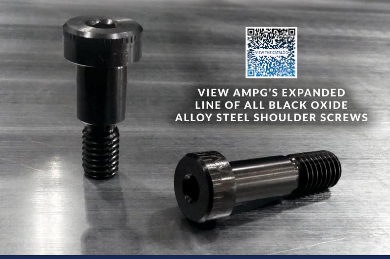
All Black Plating (No Ground Shoulder), Runout is 3X better than ASME B18.3 calls for, Concentricity is 7X better than ASME B18.3 calls for, USA Made, RoHs, REACH, DFARS Compliant, 140,000 Tensile, 84,000 Shear and C32 minimum Hardness.
